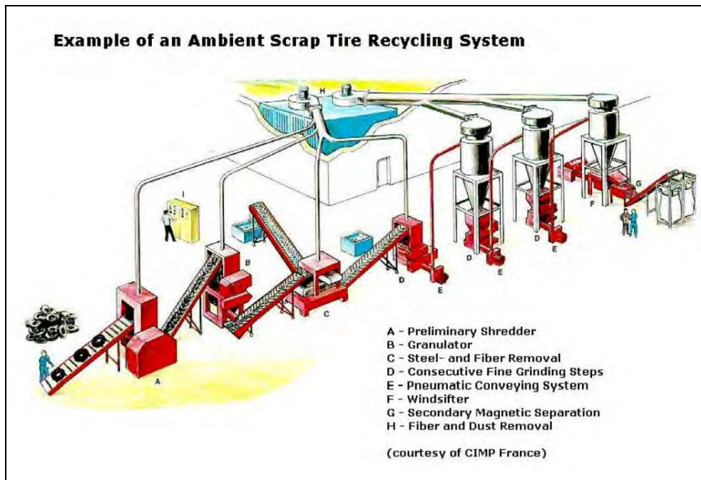
Fig. 4. Example scrap tire recycling system (courtesy of CIMP France).
