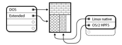
Figure 25.7. Disk Drive With Extended Partition
