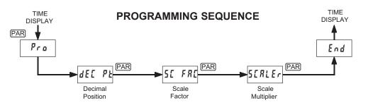
The Process Time Indicator has three programmable parameters which are entered in the sequence shown above, using the front panel push buttons.
