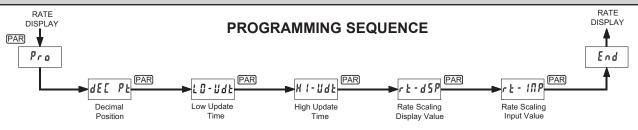
The Rate Indicator has five programmable parameters which are entered in the sequence shown above, using the front panel push buttons.
