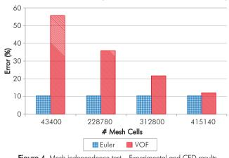
Figure 4. Mesh independence test – Experimental and CFD results comparison
