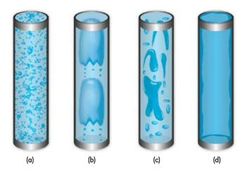
Figure 1. Flow patterns in vertical pipes. a) Bubbly & mist flow. b) Slug flow. c) Churn flow. d) Annular flow. Source: (Bratland, 2010).
