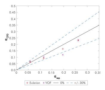
Figure 6. VOF model and Eulerian model predictions for cases A, B, C and D
