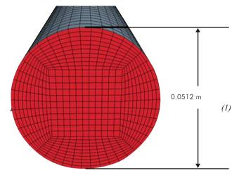
Figure 3. Orthogonal (Butterfly) grid
