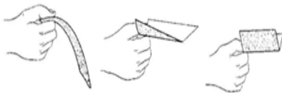
Figure-1. Form-resistant structure[1]: a/ Thin Shell b/ Folded Plate
