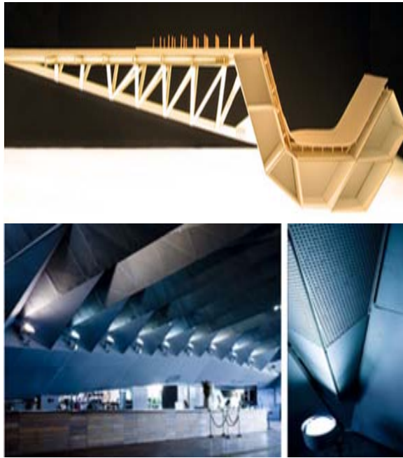
Figure-14. (top): Illustration of the steel structure [19]; (bottom): the interior (left), and the perforated ceiling detail [20] (right).
