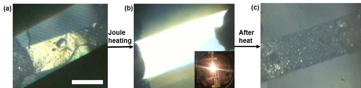
Figure S1. (a, b) Optical images of pre-annealed RGO film under current induced high temperature process. The high temperature process accompanied by a bright light, as shown in (b). Insert is the digital image taken by iphone6. (a) Scale bar represents 500 \mu\text{m} . The optical morphology of RGO film after joule heating is shown in (c).
