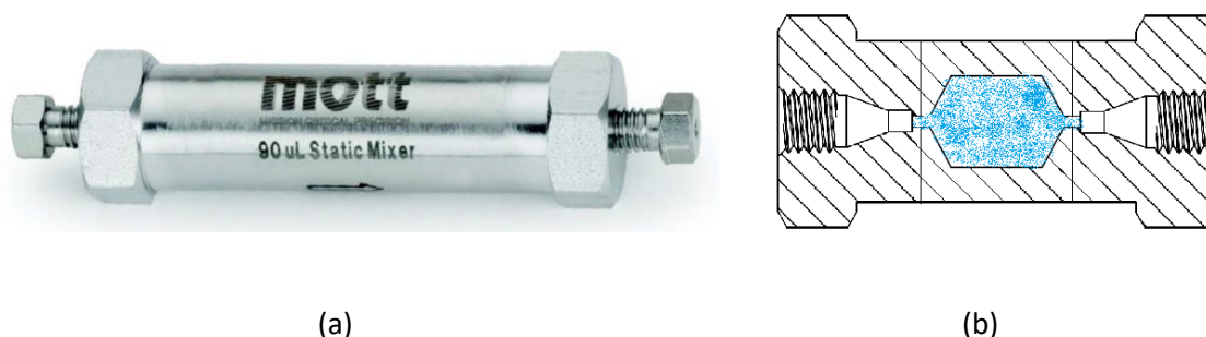
Figure 1. Photograph of a Mott 90 \mu\text{L} static mixer (a) and a schematic representation showing a cross-section view with the mixer fluid flow path shaded in blue (b).
