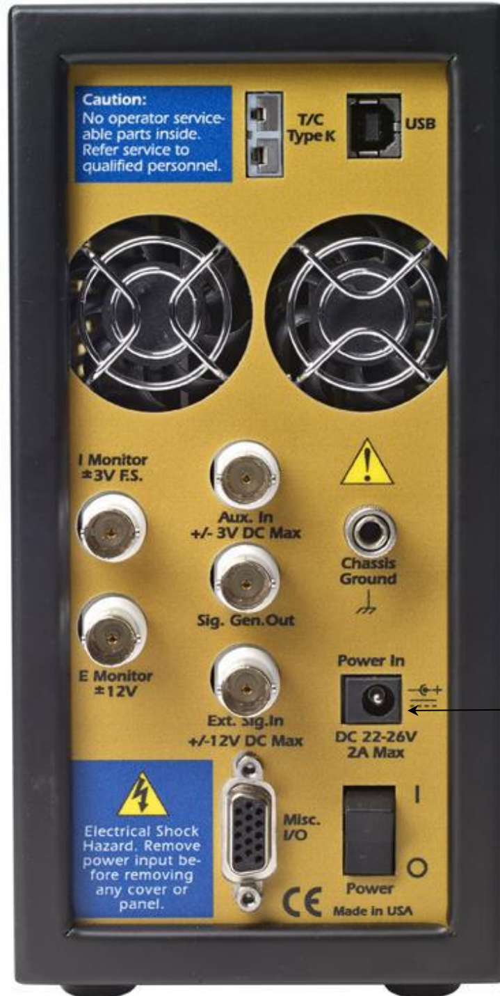
Figure 4-2 Rear Panel of the Reference 600+
