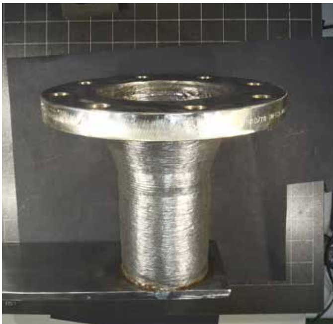
Ti6Al4V-WAAM-parts developed at Idonial workshop
