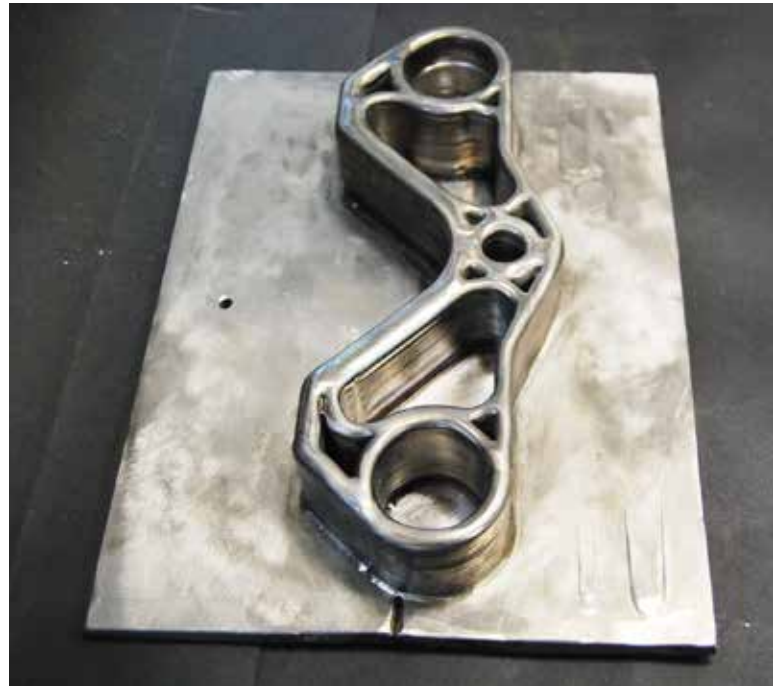
Ti6Al4V-WAAM-parts developed at Idonial workshop
