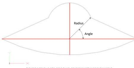
FIGURE 7 TOOL PATH OF POLAR COORDINATE MODE EXAMPLE
