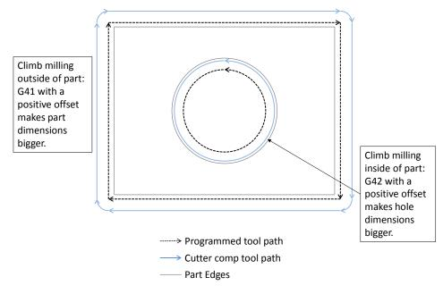
Figure 41-2: Cutter compensation OD and ID features. FIGURE 29 CUTTER COMPENSATION OD AND ID FEATURES
