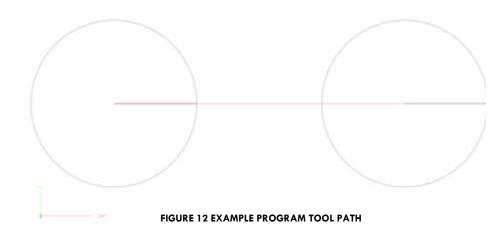
Once set, the setting will remain until cancelled by another G52 or the system is reset. As in the example above, a local coordinate system can be cancelled by specifying the axis with a value of zero. This effectively sets the local coordinate system shift to zero, giving it no effect.
