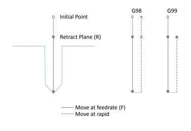
Figure 98-1: Initial and R point return setting.
