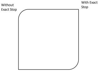
FIGURE 5 SQUARE WITH EXACT STOP ON TWO CORNERS
