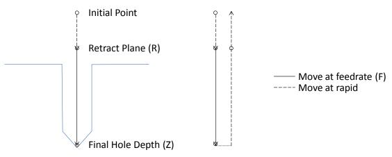
FIGURE 18 MOTION OF TOOL POINT FOR G81 CYCLE. END Z POSITION WILL BE DETERMINED BY G98/G99 SETTING
