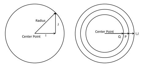
FIGURE 6 TOOL MOTION DURING CIRCLE INTERPOLATION
