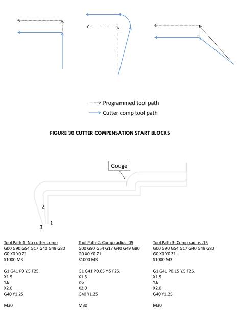
FIGURE 31 CUTTER COMENSATION RADIUS AND GOUGE
