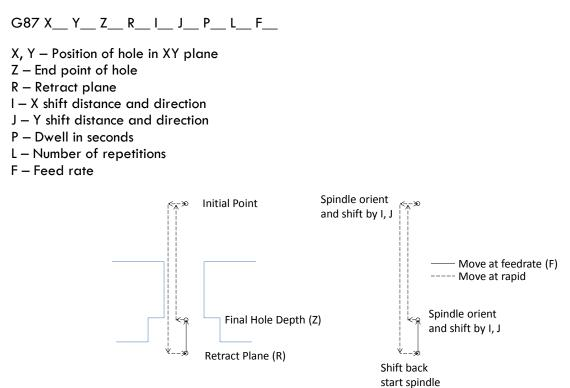
FIGURE 25 MOTION OF TOOL POINT FOR G87 CYCLE. END Z POSIITON WILL BE DETERMINED BY G98/99 SETTING
