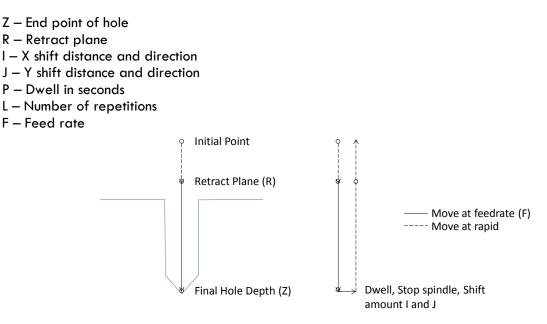
FIGURE 22 MOTION OF TOOL POINTFOR G76 CYCLE. END Z POSITION WILL BE DETERMINED BY G98/99 SETTING
