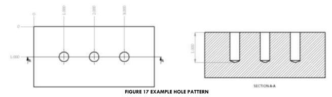
**G80 – Canned Cycle Cancel:** To end a canned cycle a G80 must be called. G80 should be specified on its own line to avoid any unintended movements. For example:
