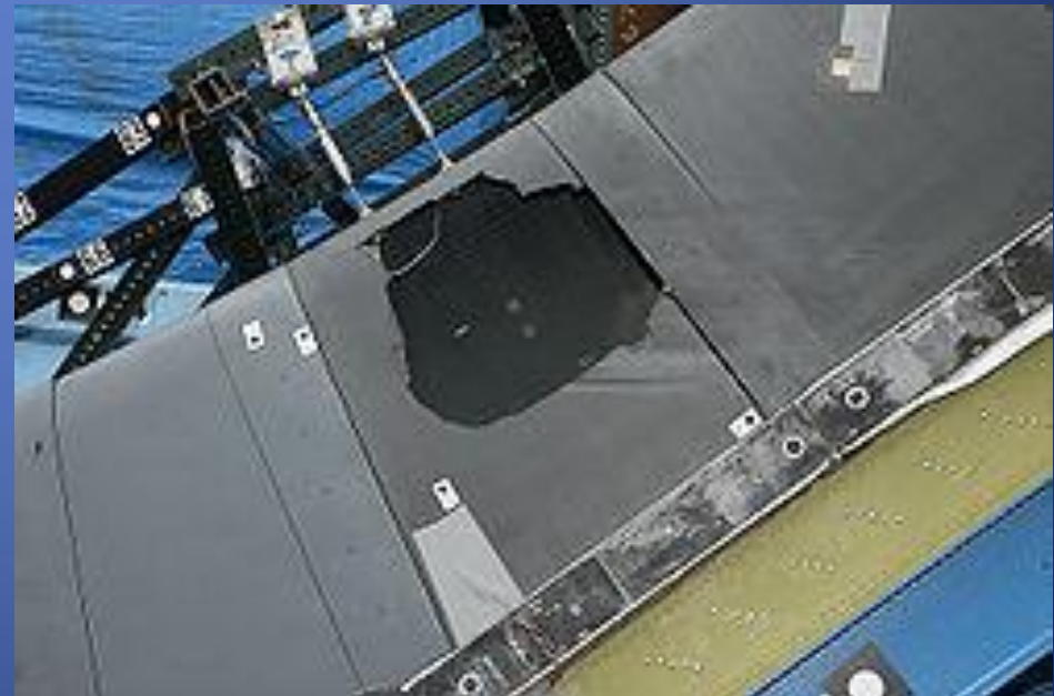
RCC panel foam impact test
