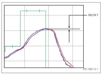
Figure 3-1 Identification of Temperature Delta at Peak Reflow Temperature
