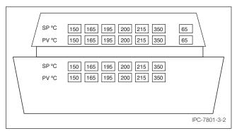
Figure 3-2 Example of Reflow Oven Recipe Set Points SP = Set Point
