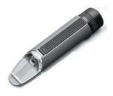
Dissolved sugar changes the refractive index of water substantially. Since sugar is the primary ingredient in juices, the "Brix" scale of refractive index was developed.
