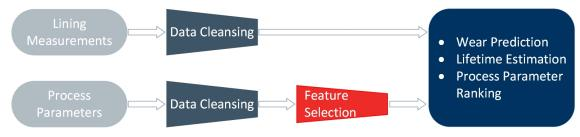
Figure 3: Data processing pipeline for wear prediction.
