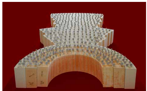
Above: Blast furnace bottom segment
