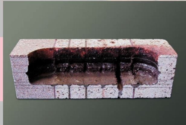
Above: Abrasion and slagging analysis of the refractory materials.
