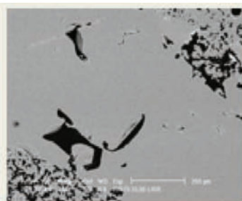
Figure 1: Microstructure of White Fused Alumina
