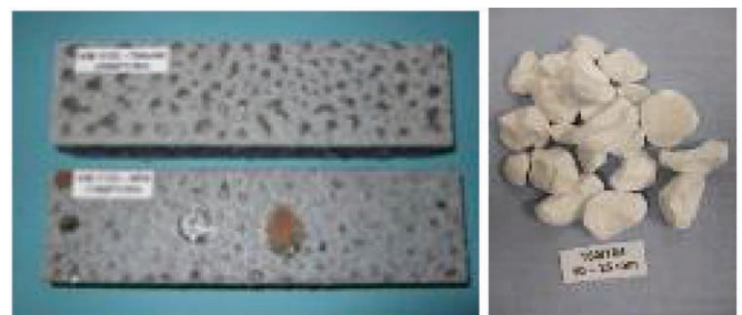
Figure 4: Pre-fired trough castable bars with tabular alumina and brown fused alumina; Almatix coarse Tabular Alumina 10-25mm
