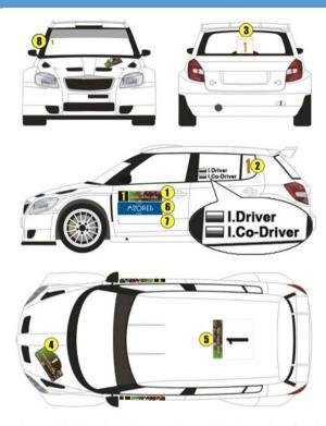
DOOR PANELS (1) - Each panel shall be placed horizontally at the leading edge of each front door with the number at the front. The top of the panel shall be between 7 cm and 10 cm below the lower limit of
