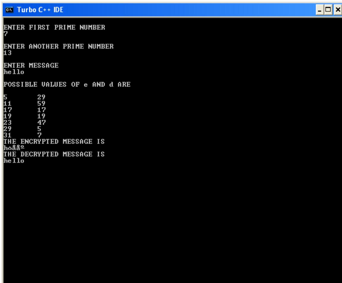
A screenshot of the Turbo C++ IDE window. The title bar reads "C:\ Turbo C++ IDE". The main window area is black with white text. The text shows the execution of an RSA encryption program. It prompts for two prime numbers (7 and 13), a message ("hello"), and lists possible values for e and d. It then displays the encrypted message "hΔ&&e" and the decrypted message "hello".
