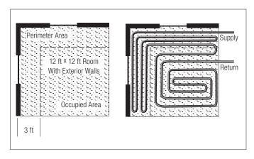
Fig 6.4: Overpour with perimeter and occupied areas using one circuit
