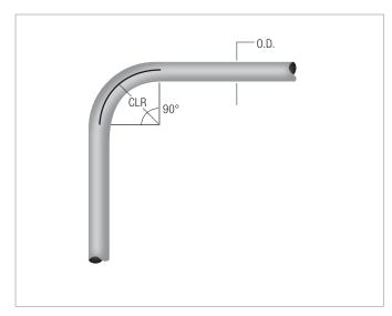
Fig. 4.3: Centerline radius (CLR) of RAUPEX pipe
