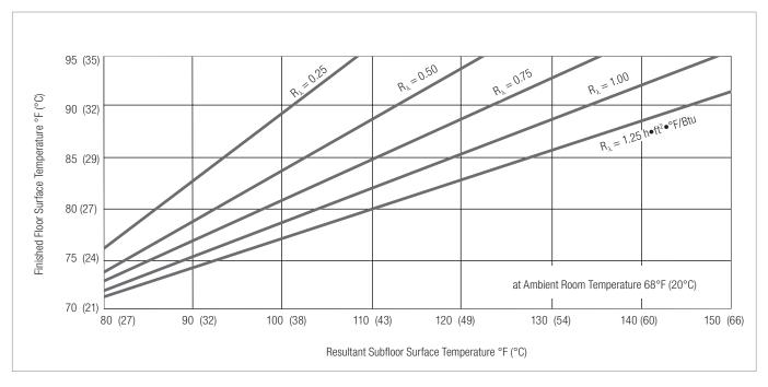
Fig. 6.1: Resultant subfloor surface temperature
