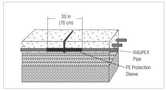
Fig. 5.6: Protective sleeving through movement joint
