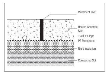
Fig. 5.2: Movement joint the pipe resulting in leaks and operational failures.
