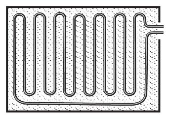
Fig. 6.7: Serpentine pipe layout
