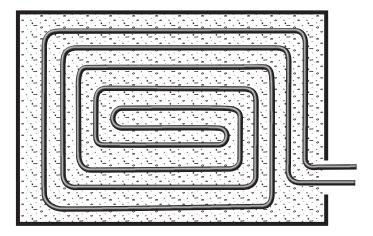
Fig. 6.6: Counter flow spiral pipe layout
