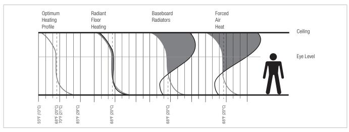
Fig. 3.1: Optimum heating distribution compared to representative temperature profiles for radiant, baseboard and forced-air heating.
