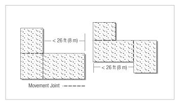
Fig. 5.4: Location of thermal mass joints mon causes of damage to thermal mass floors.
