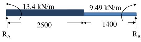
$R_A = 29.56 \text{ kN}$   $R_B = 17.22 \text{ kN}$ Shear force,  $V_{ED} = 29.54 \text{ kN}$
