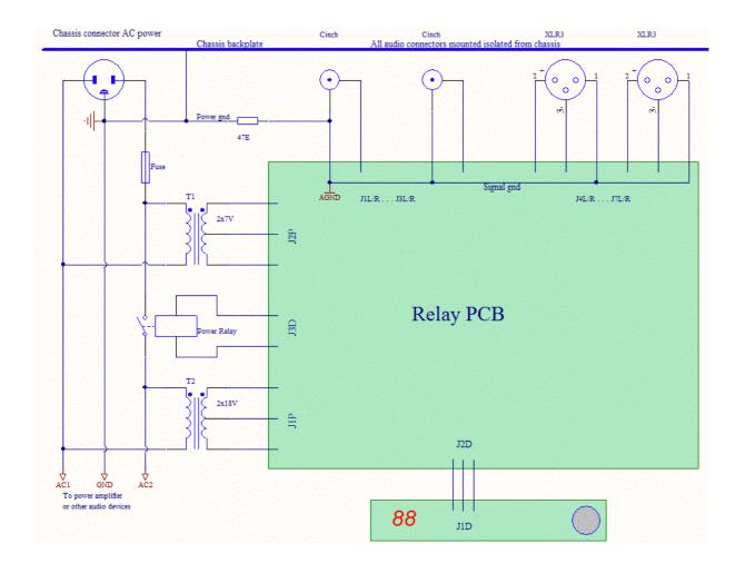
If you intend to switch a heavy transformer of a power amplifier, it is probably a good idea to add a 'varistor' across the primary side of the transformer. A varistor will prevent that switching-off the transformer creates a high-voltage arc across the relays contacts. The varistor will thus help in maintaining a proper lifetime of the relay. In any case, I would select a significantly over-powered relay, to obtain a trouble-free and very long lifetime.
