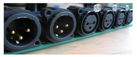
If you want to equip the preamp with 3 pair of XLR inputs plus 3 pair cinch inputs, diode D4D should NOT be mounted. Alternatively, if you want 2 XLR inputs and 4 cinch inputs, do insert D4D, and connect the 4<sup>th</sup> cinch pair to the pins marked with '+' on J4L and J4R.
