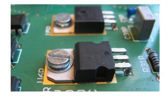
As exception to the 'normal' mounting order, prior to mounting the 4 op amps and the 2 micro controllers: complete all mounting except these 6 IC's and the XLR connectors. We can now first test the correct operation of the power supplies before inserting these IC's, avoiding the risk to blow them due to some earlier mistake. So, without the 4 op amps and 2 micro controllers U1D and U2D, you connect the two transformers, and power them up. Now the following voltages must be checked:
