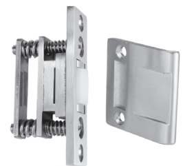
1894 Extended Cast Strike = 2-1/8" x 2-1/4" Roller latch face = 1" x 3-3/8" Maximum roller projection = 5/16"
