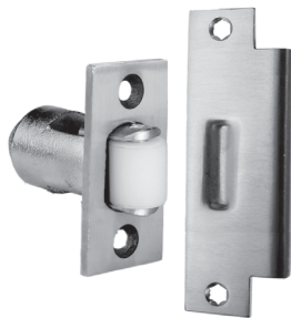
1896 ASA Strike = 1-3/8" (lip to center) x 4-7/8" Roller latch face = 1-1/8" x 2-1/4" Maximum roller projection = 1/2"
