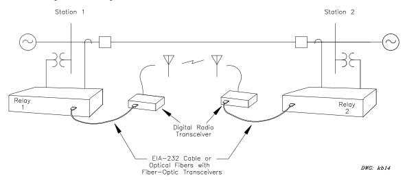
Figure 17: Digital Communication via Point-to-Point Digital Radio
