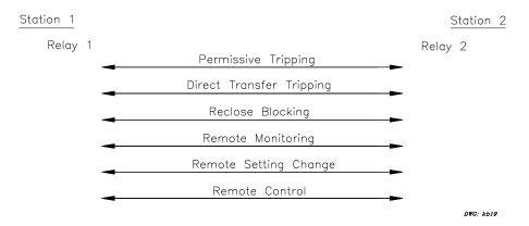
Figure 14: Summary of Relay-to-Relay Logic Communication Example
