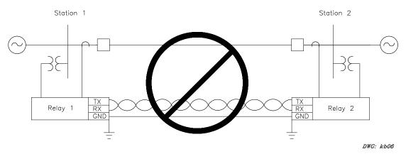
Figure 20: Direct Digital Communication via Metallic Cable - Not Recommended for Pilot Scheme Communication
