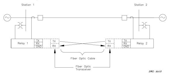
Figure 15: Direct Digital Communication via Direct Fiber-Optic Cable
