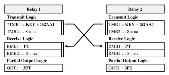
Setting TMB1 bit to KEY is equivalent to connecting a Zone 2 overreaching relay output contact to the keying input on a communication device. Likewise, assigning RMB1 to PT is equivalent to connecting the communication device output contact to a permissive trip input in the relay scheme. In this example, relay output contact OUT1 is connected to trip the local breaker when relay three-pole trip logic (3PT) asserts.
