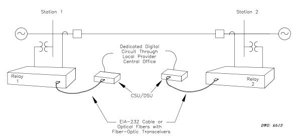
Figure 18: Digital Communication via a Leased Digital Communication Channel
