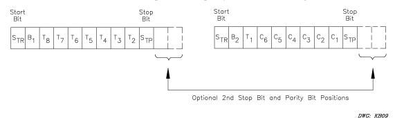
Figure 9: Asynchronous Message Framing Bits
