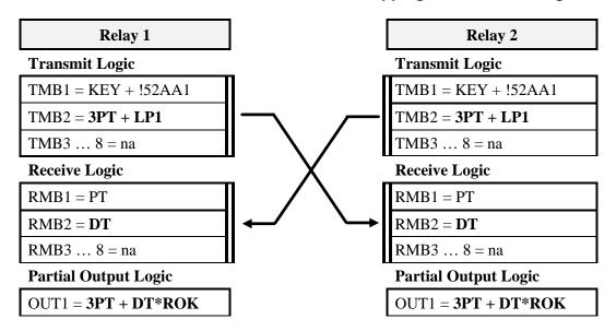
Table 2: POTT Plus Direct Transfer Tripping Pilot Scheme Logic
