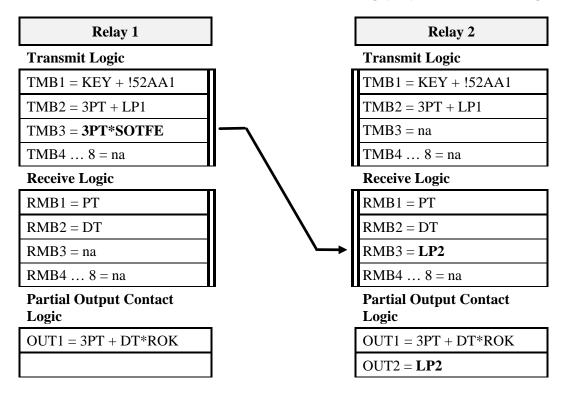
Table 3: POTT Plus DT Plus Reclose Blocking (RB) Pilot Scheme Logic
