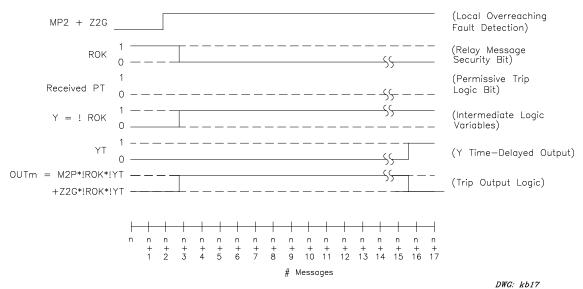
Figure 11: Relay Logic Technique for Dependable Pilot Scheme Applications
