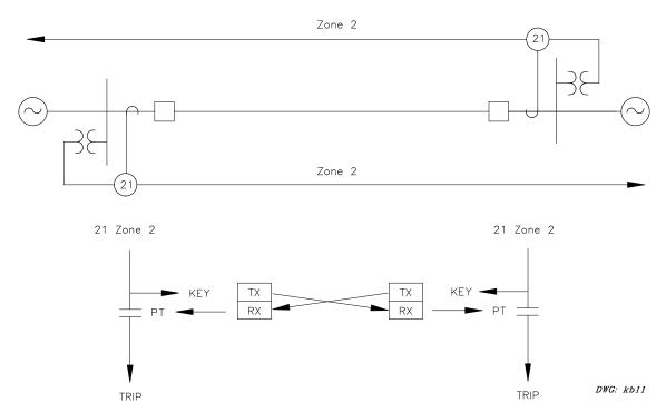
Figure 13: Basic Permissive Overreaching Transfer Tripping Pilot Communication Scheme
