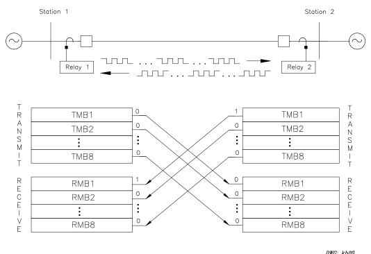
Figure 6: Relay-to-Relay Logic Communication
