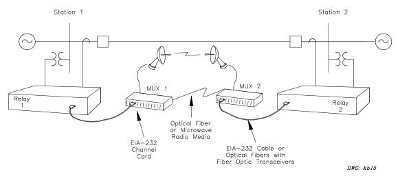
Figure 16: Digital Communication via Network Communication Multiplexers
