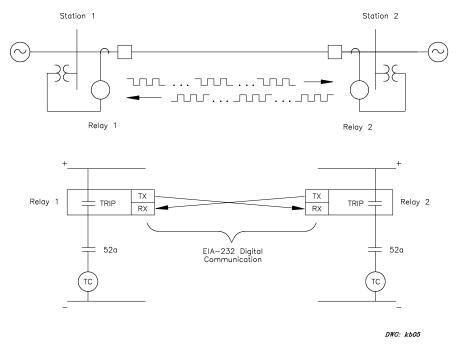
Figure 5: A New Approach: Direct Relay-to-Relay Digital Logic Communication
