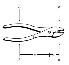
Pliers multiply the force of a person's grip through the use of leverage. For the pliers shown, A = 10 lbs., a = 3 in., and b = 1 in. What is the gripping force, B, at the jaws of the pliers?
