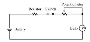
In this circuit, a potentiometer is used to control the light output of a bulb. Which of the following is the source in this circuit?
