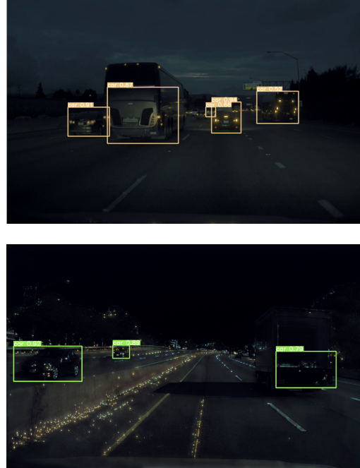
Figure 6. Predictions of bounding boxes for big vehicles from YOLOv5 model that was trained on real day images only, and tested on real night image (top) and GAN night image (bottom). In both cases, similar error patterns (lower half of truck is detected as cars) are observed.
