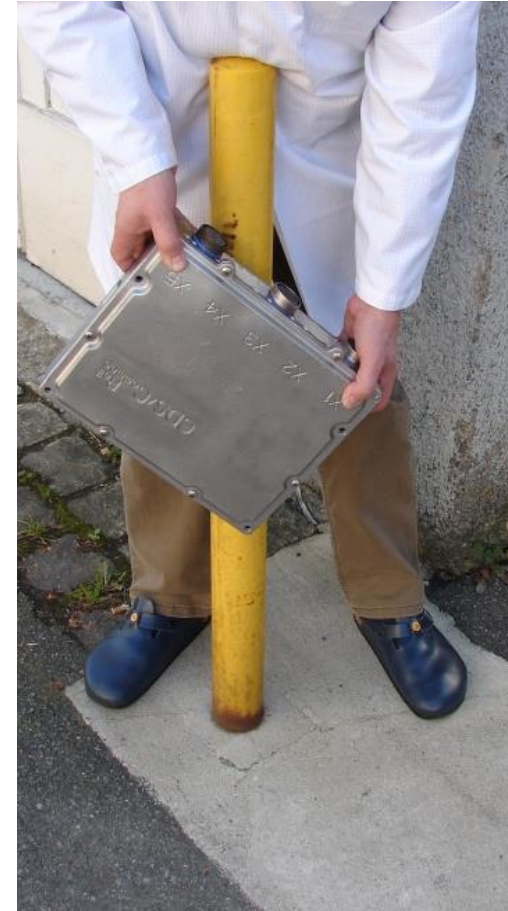
Falling Test from 50cm height on concrete slab
