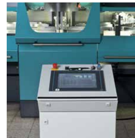
Free standing control panel for the ergonomic set-up in front of the machine.
