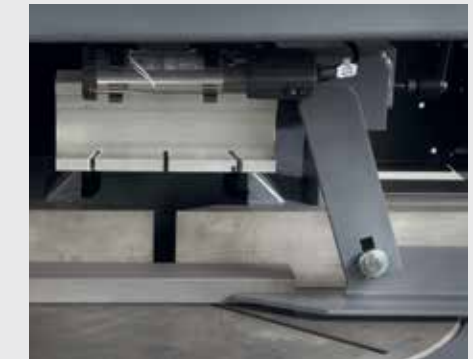
Horizontal clamping device on the removal side for material clamping during sawing.
