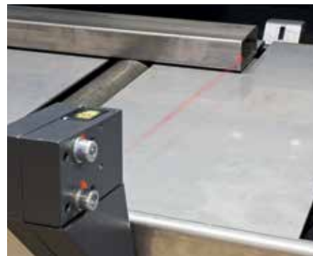
Laser light barrier for the cut identification.
