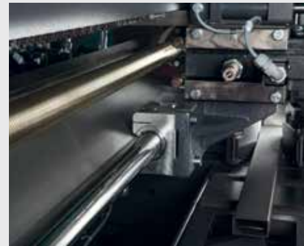
Automatic material supply via ball screw.
