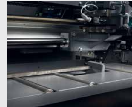
Mechanical cut stop for material identification.
