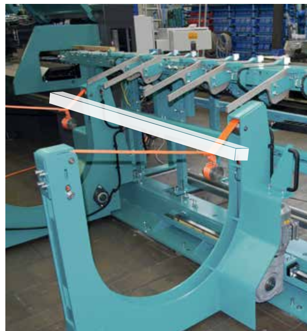
3 Automatic lowering belt troughs for the support of sections.
