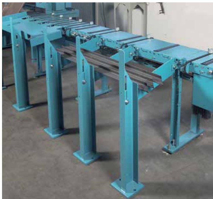
2 Section cross distributor with cross beating chains for automatic sorting of cuts forwards and backwards.
