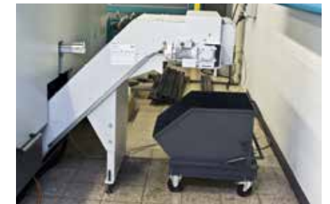
Slat-band chain conveyor for the automatic removal of swarf, cuts/remnants and gussets.
