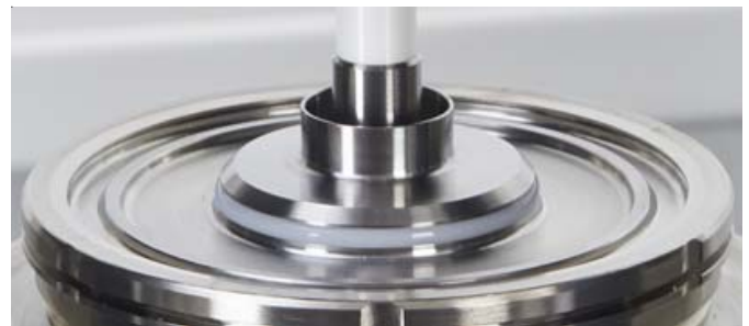
Figure 7: Lower measuring plate TMP with a diameter chosen to match the upper geometry.
