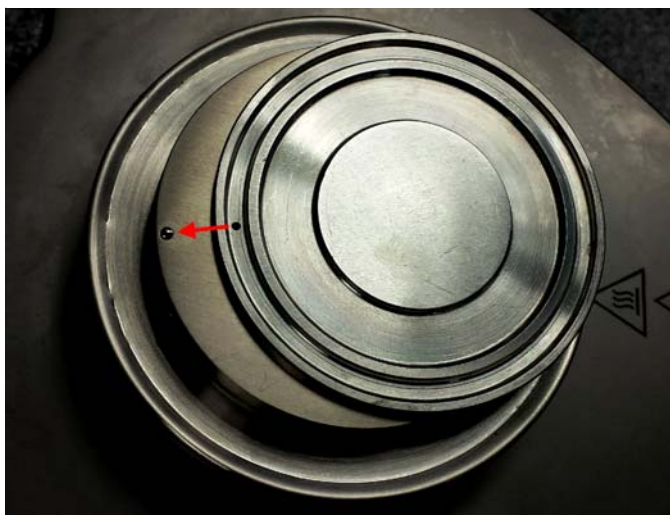
Figure 2: For our PP- and CP-geometries, measuring plates TMP with the corresponding diameters are available. The notch under the mark on the TMP slides over the pin in the temperature control unit for easy and precise positioning.
