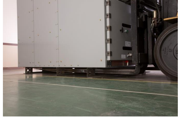
Figure 4: Complete fork penetration of all 3 shipping channels
