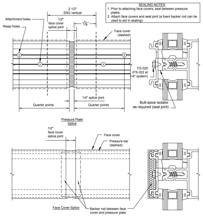
Figure 21 Pressure Plate/Face Cover Splicing & Sealing at SSG Mullions (Intermediate Horizontal Shown; Head & Sill Similar)
