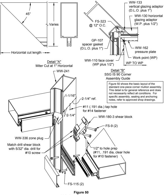
Figure 50 SSG IS 90 Corner Assembly (Cut lengths in parentheses)
