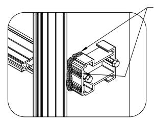
Seal face, top, bottom, and screw tracks of shear blocks.
