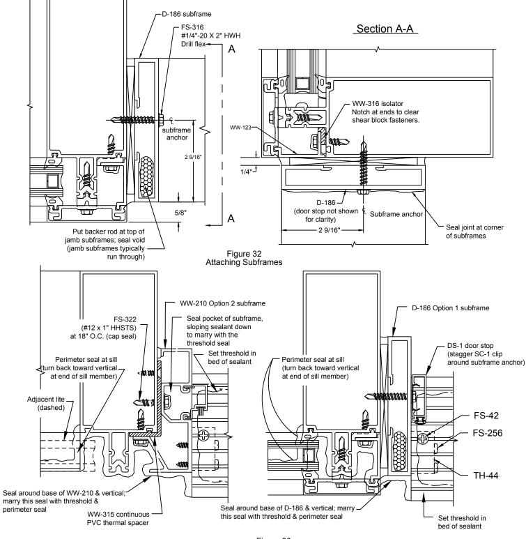
Figure 33 Sealing Verticals at Entrance Doors (Temporary Glazing Retainer Not Shown for Clarity)
