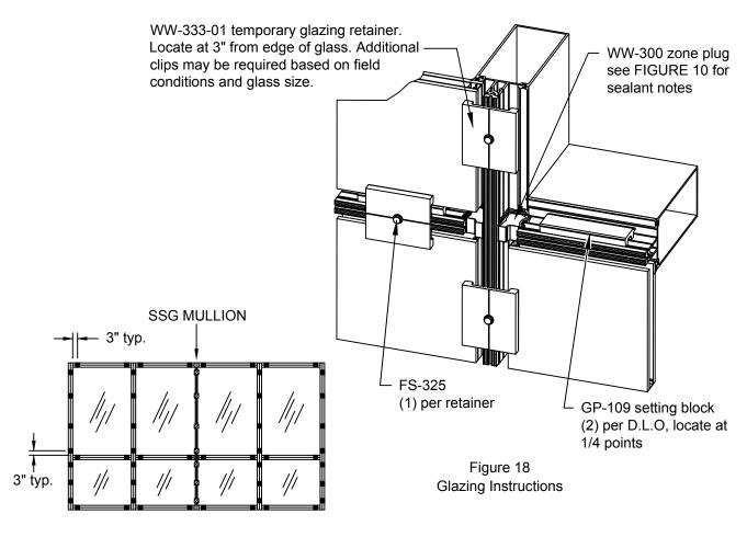
Figure 19 Typical Location of Temporary Glazing Retainers
