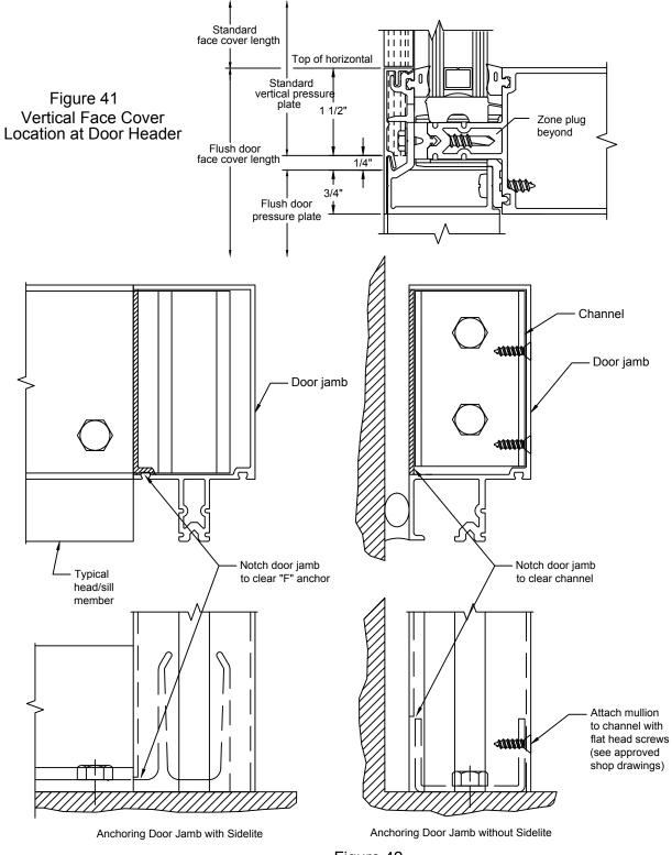
Figure 42 Anchoring Door Jamb Mullions
