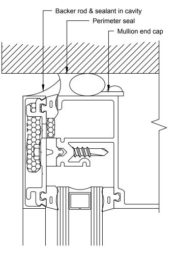
Figure 22 Sealing Top of Captured Verticals
