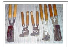
Bullet molds from left: Hensley & Gibbs with 4 cavities of 180 grain bullets for .44 Special (#271, my design); two Lee molds; a Lachmiller mold for .45 ACP; and a Hensley & Gibbs with two cavities of 158 grain SWC .358" (#73BB) and two cavities of 210 grain .430" bullets (#271BB, my design) for the .44 Magnum. There wasn't room in the photo for all my Lyman single cavity rifle molds.
