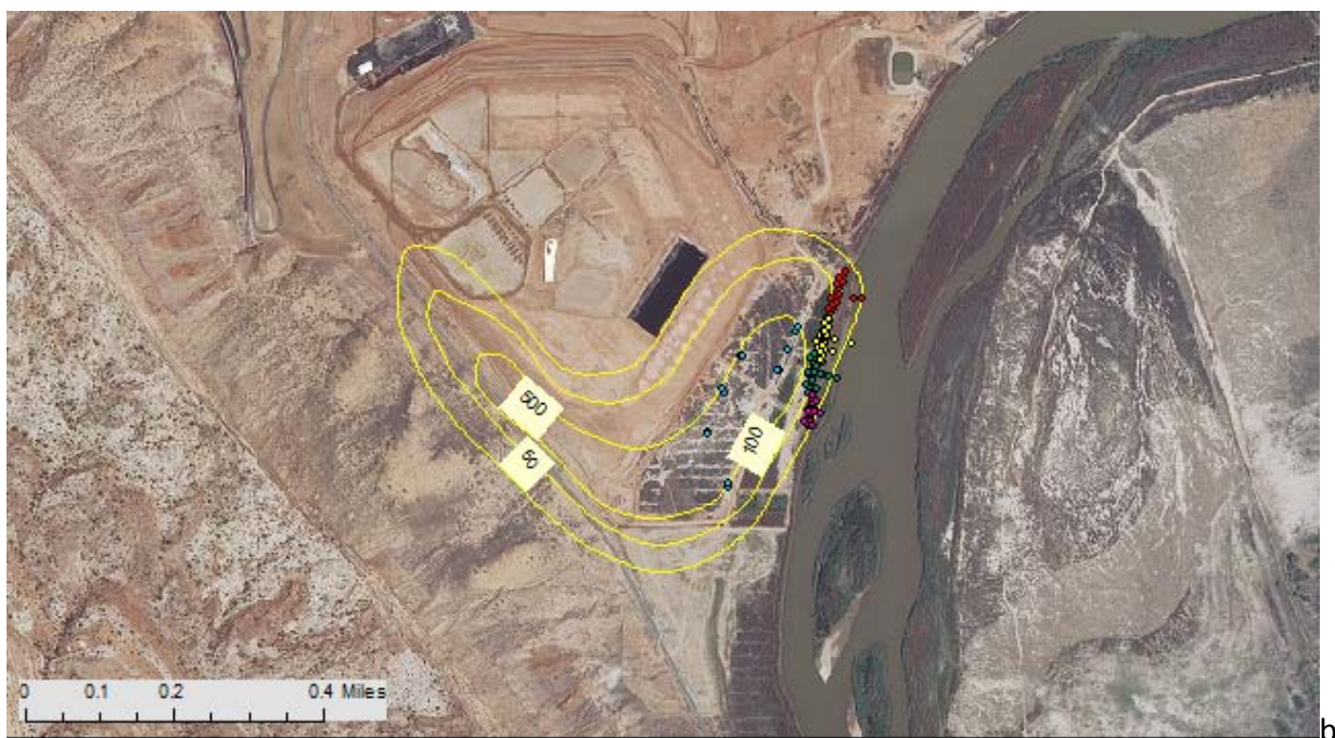
Figure 25 Ammonia (total as N) Concentrations Interpolated on the Upper Surface of the Ground Water a) June 2003 and b) October 2010
