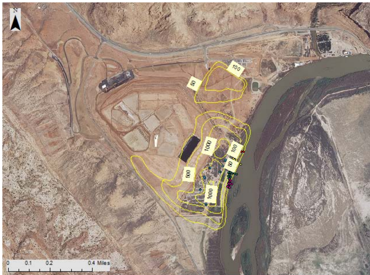
Figure 26 Ammonia (total as N) Concentrations Interpolated at 50 ft Below the Surface of the Ground Water
