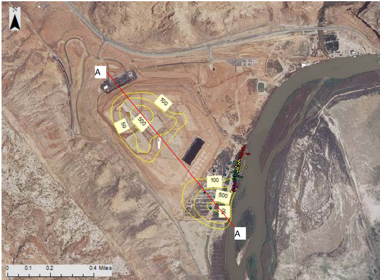
Figure 27 Ammonia (total as N) Concentrations Interpolated at 150 ft Below the Surface of the Ground Water (Section A-A is on the next figure)
