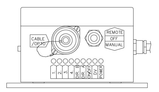
When the control unit is <u>activated</u> and the electronicbox switch is in "REMOTE" position do any of these LED combinations exist?
