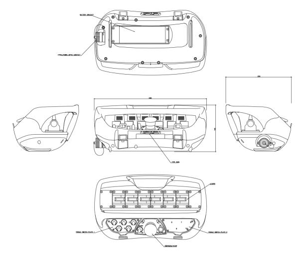
Portable control unit <u>with</u> battery operation ( radio control or opto fibre cable ). A battery is located in the control unit for radio control and is very simple to change.
