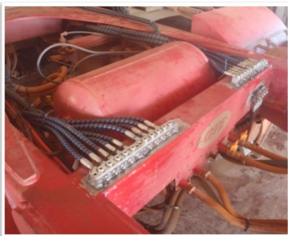
4 x 5 outlet grease anchor blocks and 8.6mm high pressure hose on truck dollies
