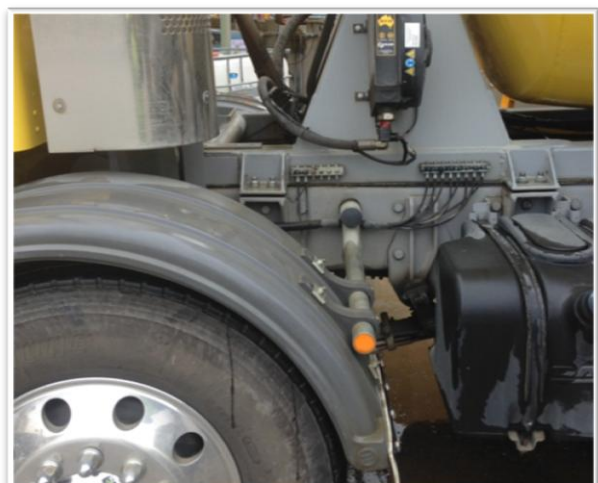
2 x 6 outlet grease anchor blocks and 6mm nylon tube on cement truck
