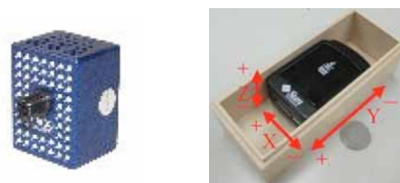
(a) 3D distance image sensor (b) Wireless sensor device Fig.6. Measurement system for human behaviors
