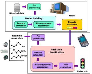
Figure 1. Components of a real-time physiological alerting system. (Apiletti, et al., 2009)
