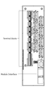
Remote Power Panel with input and output breakers (PBK8-40-13-10-CE)
