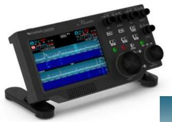
A FlexRadio Maestro (wireless or wired) connects across a local network or the internet to control a FlexRadio station. Can also control from a PC program or App on smartphone or tablet. Remote access is "built-in" to the SmartSDR software.
