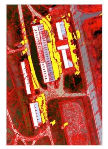
Figure 4 | Rule-based classification of shadow for Goshen data (yellow represents shadow)
