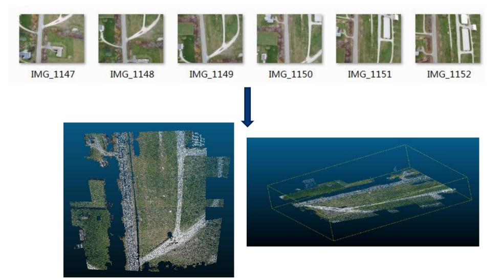
Figure 7 | Cloud point data generated from OpenDroneMap
