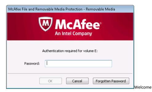
If the autorun script program does not force the login screen to appear, you may run the MfeEERM.exe program in the root directory of the flash drive. Enter the password for the USB key and access will be granted.
