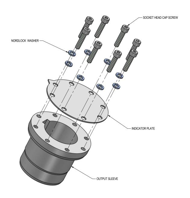
TYPICAL EXPLODED VIEW OF INDICATOR PLATE, OUTPUT SLEEVE AND OUTPUT SLEEVE SCREWS
