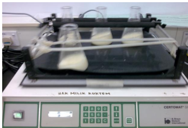
Figure 3.4: Orbital shaker that use to shake the solution
