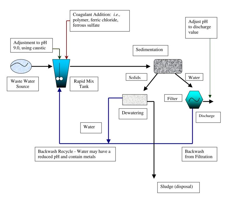
Figure 8 - The Processes of a Conventional Metals Precipitation Treatment Plant
