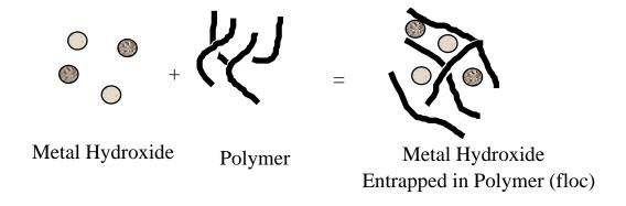
Figure 9 - Aggregation of Metal Hydroxides.
