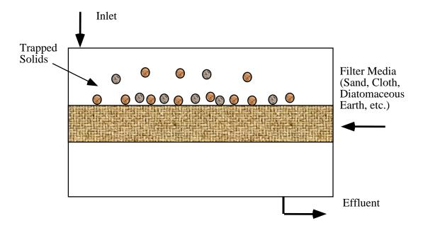
Figure 11 - Filtration Unit for Metals Removal.
