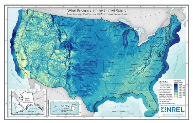
Figure 12. Wind resource in the CONUS at 100 m above the ground Image is from (Draxl, Hodge, Clifton, & McCaa, 2015).
