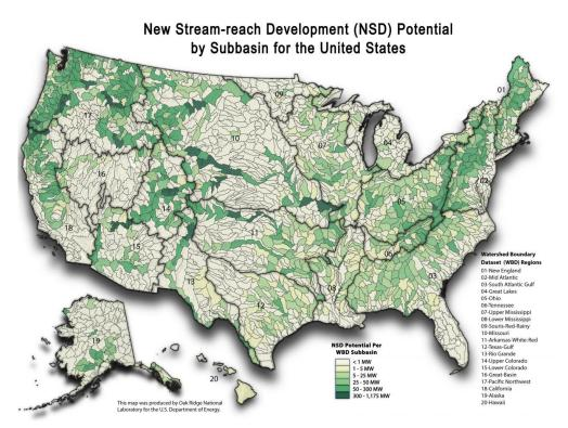
Figure 35. Map of new stream-reach development resource potential by subbasin for the United States Image is from (McManamay, et al., 2014).
