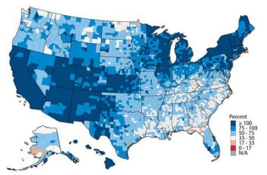
Figure 7. Percentage of low-to-moderate income household electrical consumption that can be offset by rooftop solar generation considering all low-to-moderate income residential building stock
