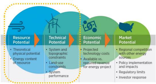
Figure 1. Differences in four common potential assessment calculations
