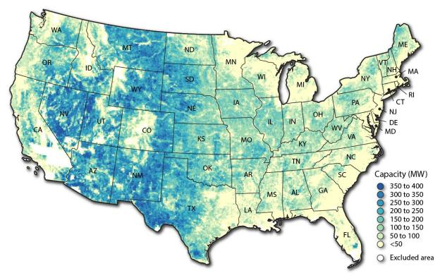
Figure 13. Technical capacity potential for land-based wind across CONUS assuming reference land restrictions Image is from (Lopez, et al., 2021).
