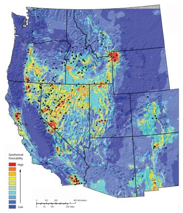
Figure 29. Map from USGS special models showing the relative favorability of occurrence for geothermal resources in the western CONUS
