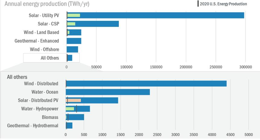
Figure 2. Annual technical energy potential for all renewable energy resources in the United States, the portion of each available within 10 mi of federally recognized Tribal lands, and historical 2020 energy production.
