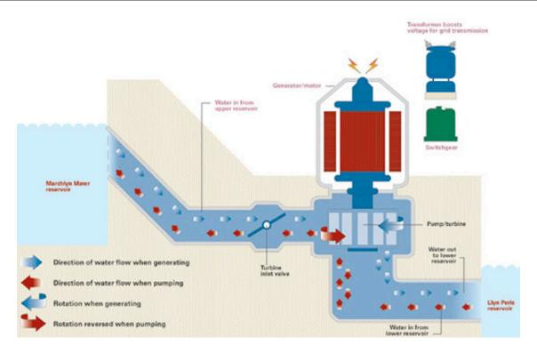
Source: International Power "The Principles of Pumped Storage," web article. http://www.fhc.co.uk/pumped\_storage.htm (accessed June 10, 2008)
