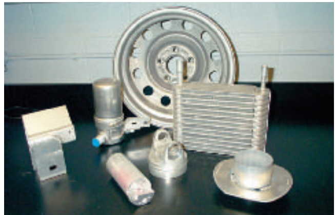
Some automotive components in aluminum that have been repaired by welding.
