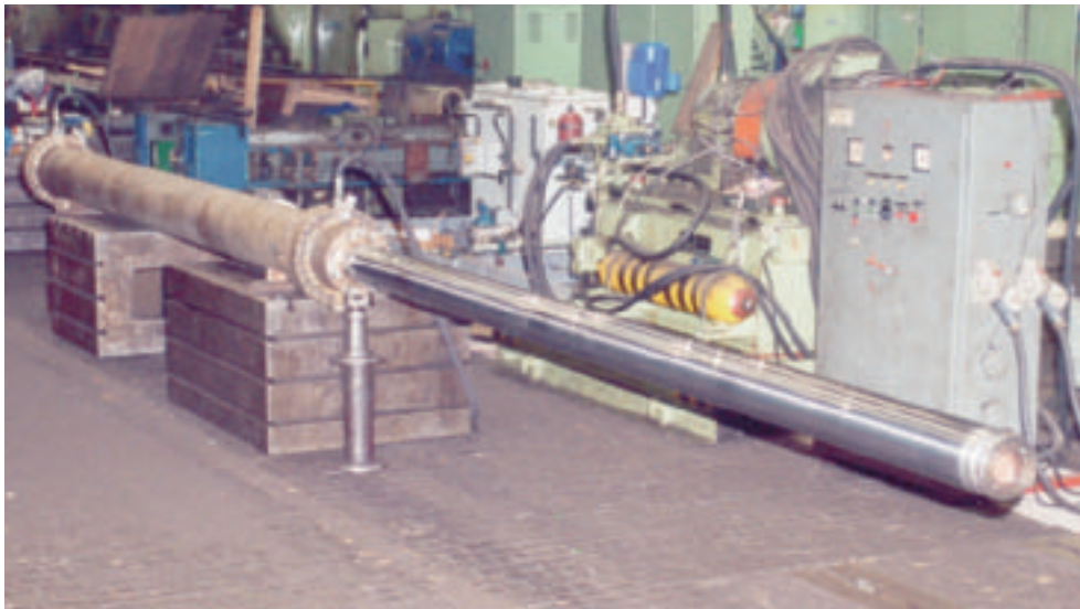
Figure 3. Piston after welding overlay and machining
