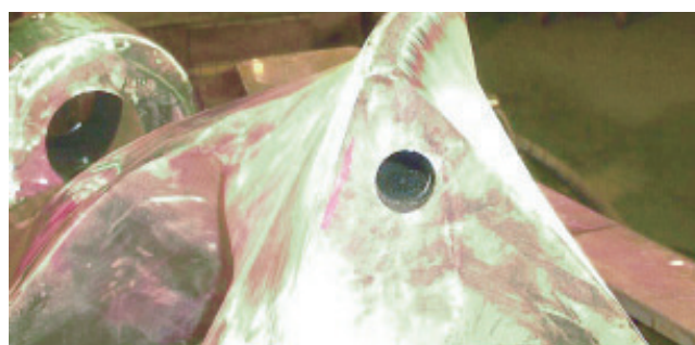
Fig. 1. First build-up layer welded on the mixer blade with OK Tubrod 15.34.
