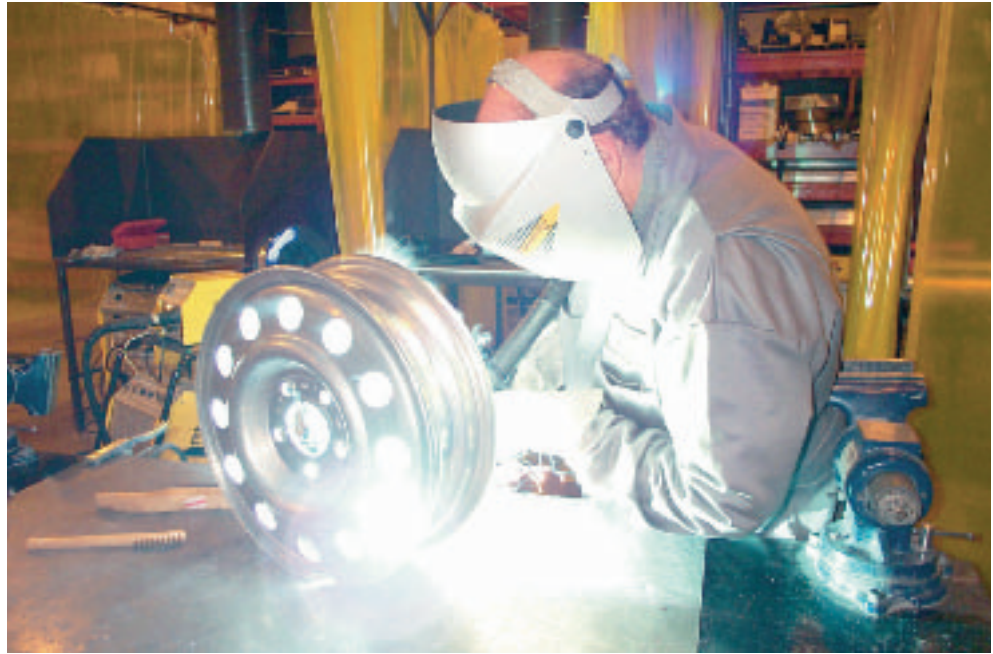
Special care should be taken when welding high performance components such as car rims.
