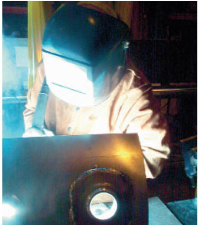
The most important consideration before repair welding is the identification of aluminum base alloy type.
