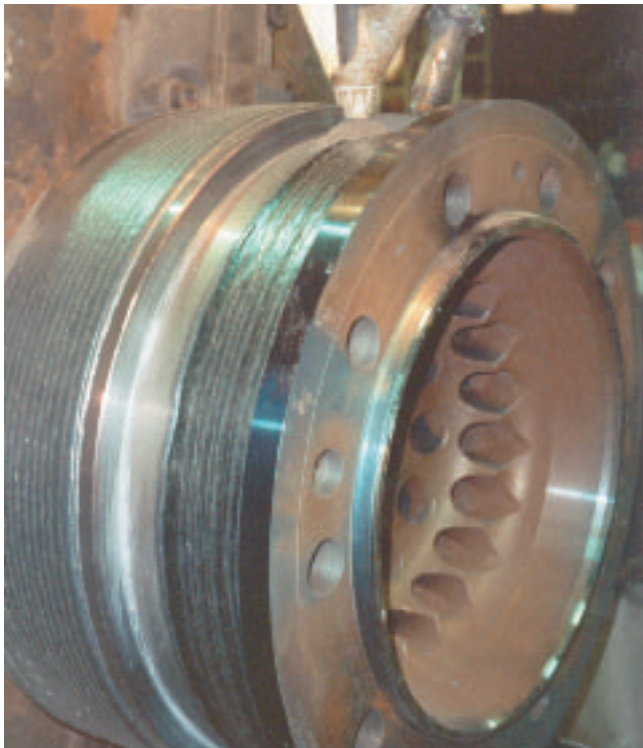
Figure 2. Today: easy handling. An increase of more than 50% in deposited weld metal
