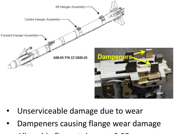
• Allowable flange tolerance 0.25 mm
