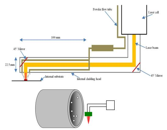
Schematic of a cladding nozzle for the internal repair, designed by Fraunhofer Institute of Laser Technology
