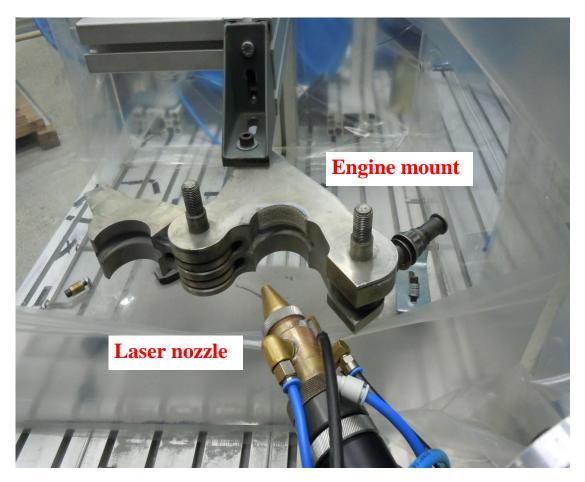
Set-up for repair at Swinburne University
