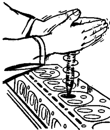
Lapping the valve and seat by hand—typical
