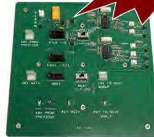
Fan Control Board w/ built in Sensors (no paddles needed)
