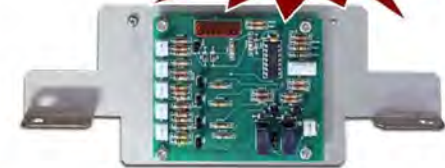
(1) # TFC-3X90ACAF-01 Fan Alarm Control Board w/ Mounting Bracket
